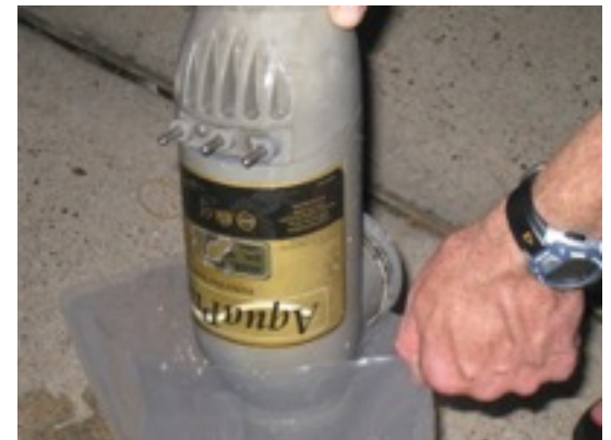
Step 6 – Remove from bag, flush contents to drain, dispose of bag and re-install
