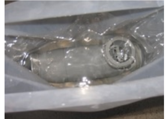
Step 3 – Add water until chlorinator is fully submerged. Do not exceed more than 1 gallon water per 32 oz. Piranha Salt Cell Cleaner.
